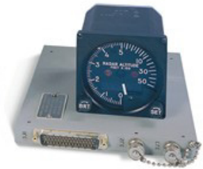
SIGNAL DATA CONVERTER (SDC)
