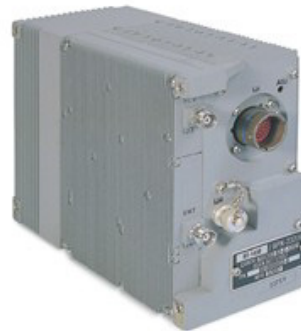
RECEIVER TRANSMITTER (RT)
