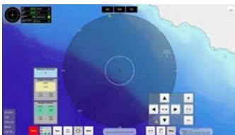
Firefly Active Continuous Wave Mode Display shows the dip point in the center and two targets being tracked. Current Sonar parameters are shown in overlays.
